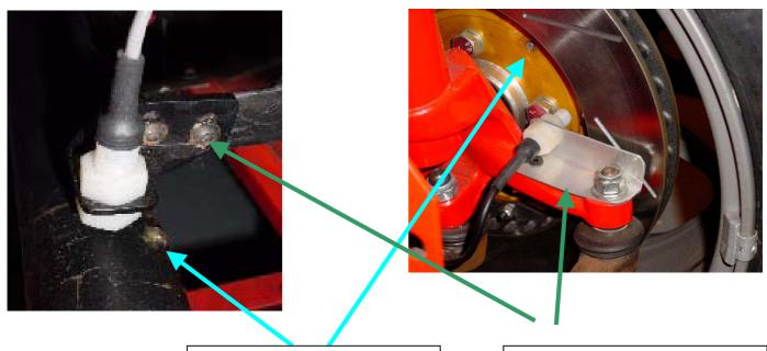
Magnets glued in position. Liberal application of a strong adhesive such as Araldite will ensure that the magnets do not become dislodged during use. Strong mounting brackets that hold the speed sensors in position. The brackets have been mounted in positions that move in unison with the magnets.
