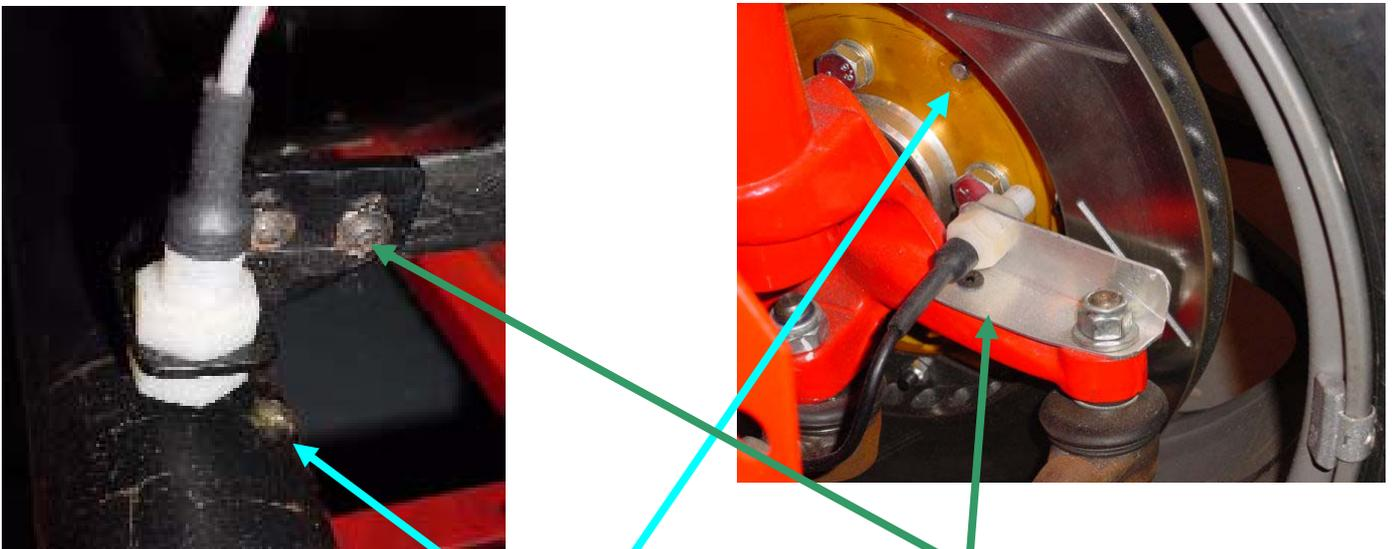
**Magnets glued in position. Liberal application of a strong adhesive such as 'Chemical Metal' or 'Araldite' will ensure that the magnets do not become dislodged during use.**
