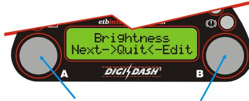
**To enter the set-up Menu, Hold Down Buttons A & B Together**
